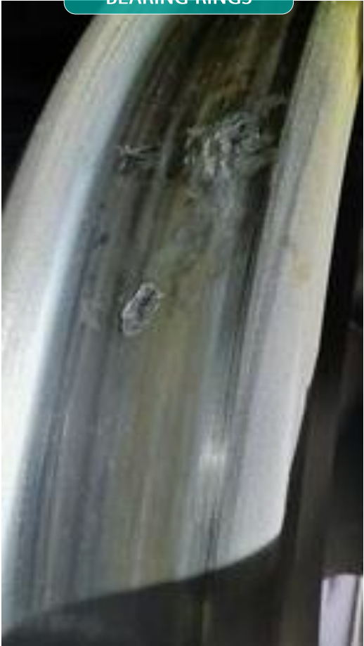
SLIGHTLY WORN BEARING RINGS ✗
